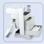
Patented modular housing design allows fast and comfortable filter replacement without tools. Independent filter stages allow each filter to be replaced individually, rather than having to replace entire filter blocks. This maximises yield and minimises replacement costs.
